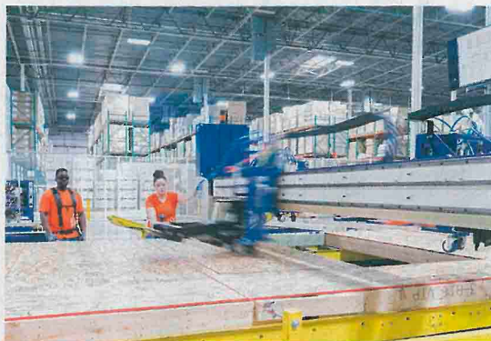
◀ At a factory in Phoenix, Kattera staffers and robots build prefab wall panels on an assembly line
