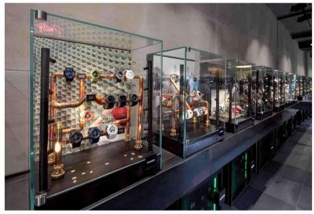
colour rendering (CRI90) and 4.000K cool white colour temperature as we felt that a cooler light source would work better with the modern finishes in the space. Finally. a fairly narrow beam angle was used so that we could create contrast in the space.' says Mark Shortland, managing director of Shoplight.
