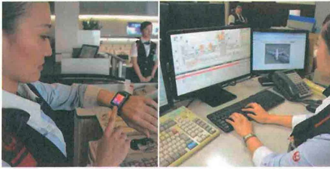
Japan Airline staff equipped with smart watches enabling the control desk tracking their whereabouts using iBeacons (source: Future Travel Experience)
